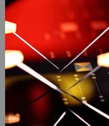
Fig. 2: Electrical characterization of sintered silver interconnects.
