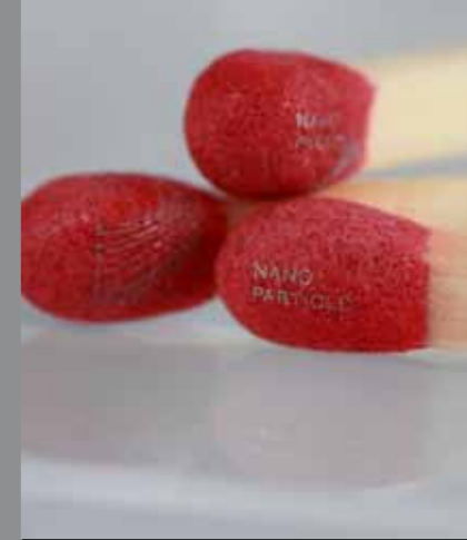
Fig. 3: Printed Ag ink on top of 3-D substrate
